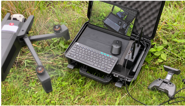
Figure 5: The video-analyzer app was ported to an Nvidia Jetson Nano platform for real-time field tests
